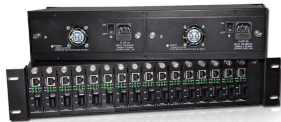
2U 19"16 Slots Rack for Card Based Media Converter
